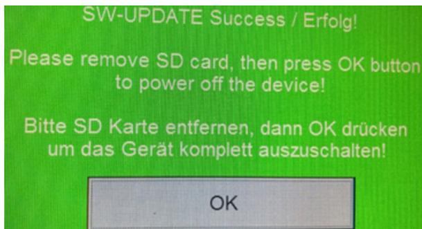
8. When the green screen that indicates the successful installation, remove the memory card and press "OK" finish the process and to power down the device
